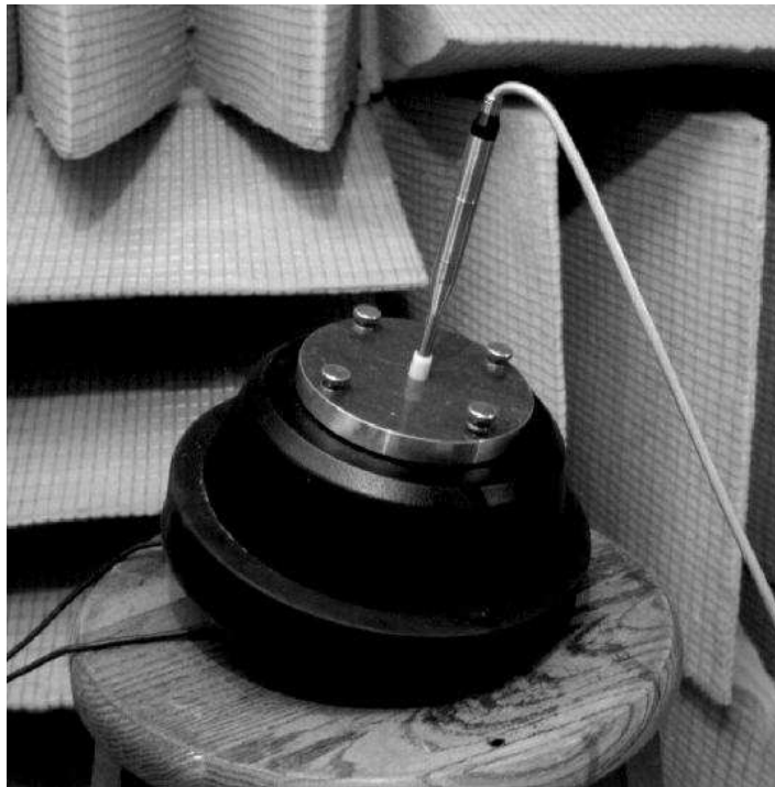
Figure 4.8: Photograph of the compression horn driver blocked for two-port parameter measurements. The B&K 1/4 in. microphone is mounted in a nylon sleeve. The aluminum blocking plate is 9.525 mm (3/8 in.) thick.
