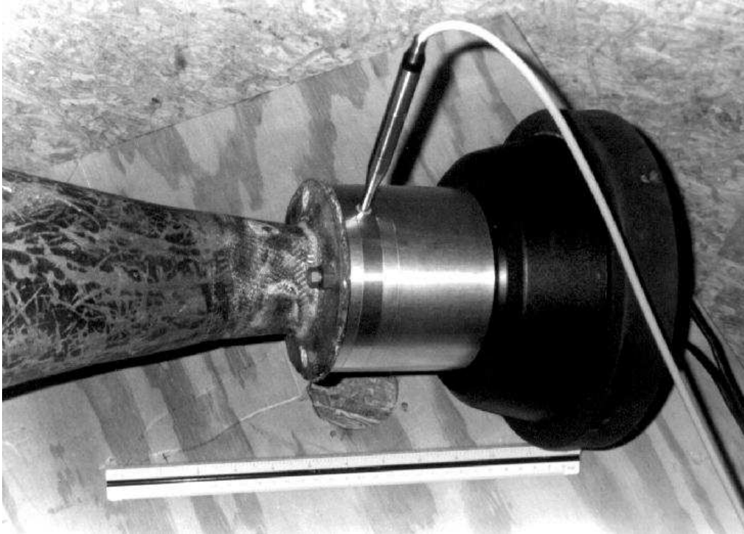
Figure 4.15: Photograph of the two-microphone measurement system showing minimal length section of standing wave tube inserted between the compression horn driver and the throat of the horn. The microphone is shown in the first of two measurement locations. The spacer between microphone and horn throat is 3/8 in. thick, the plate containing the microphone is 1/2 in. thick, the remaining section between the microphone and compression horn driver is 2\ 7/8 in. thick.
