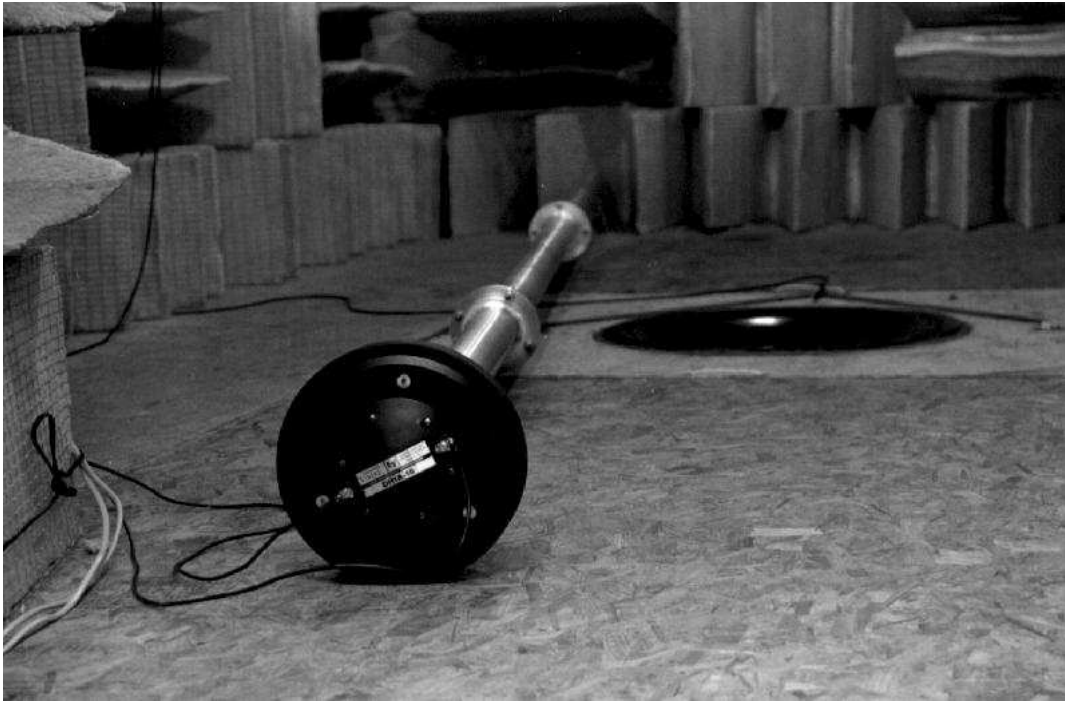
Figure 4.10: Photograph of anechoic termination used for two-port parameter measurements, A' and C' . The compression horn driver is the Electro-Voice DH1A-16. The anechoic termination is constructed from a linear taper of fiberglass in a 10 ft length of aluminum tubing. Note the horn mounted in the floor to the right of the anechoic termination.
