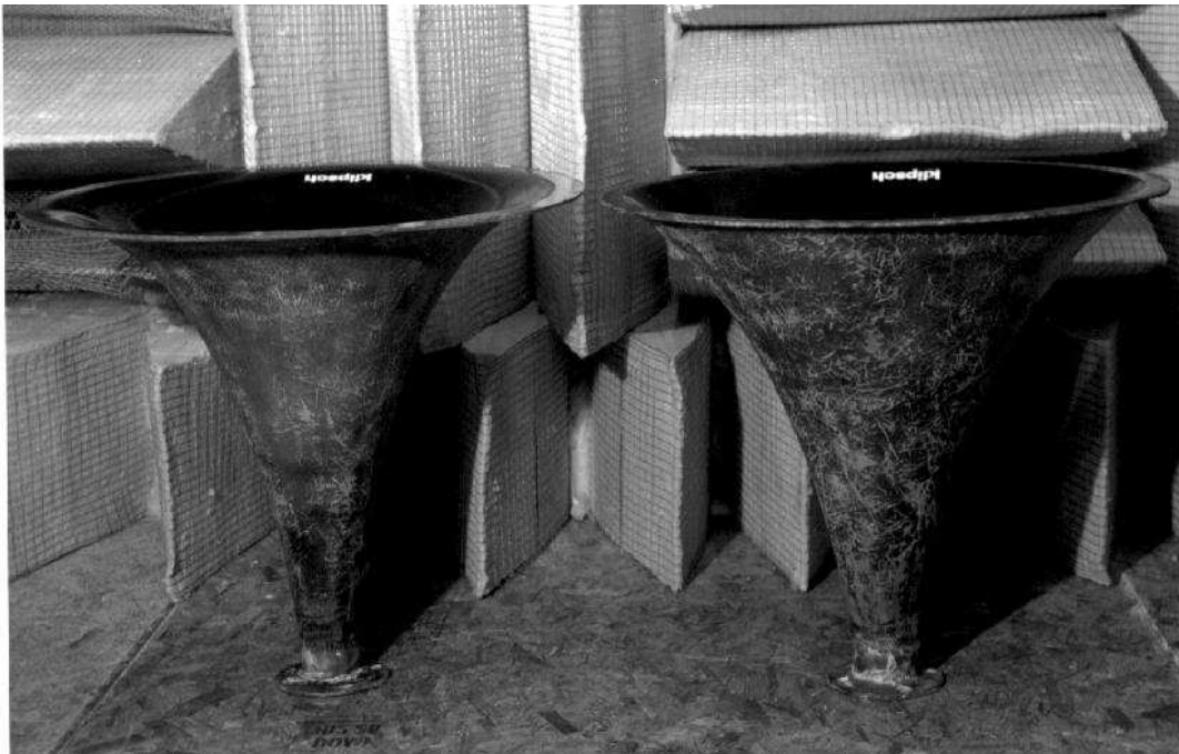
Figure 4.3: Photograph of the tractrix and exponential horns constructed for experiments. The tractrix horn is on the left and the exponential horn is on the right. Note the larger diameter of the area profile for the exponential horn. Dimensions: throat radius: 25.4 mm (1 in.), mouth radius: 271 mm (10.67 in.), axial length: 559 mm (22 in.), cutoff frequency: 232.5 Hz, exponential contour wall length: 627 mm (24.7 in.), tractrix contour wall length: 642 mm (25.3 in.)
