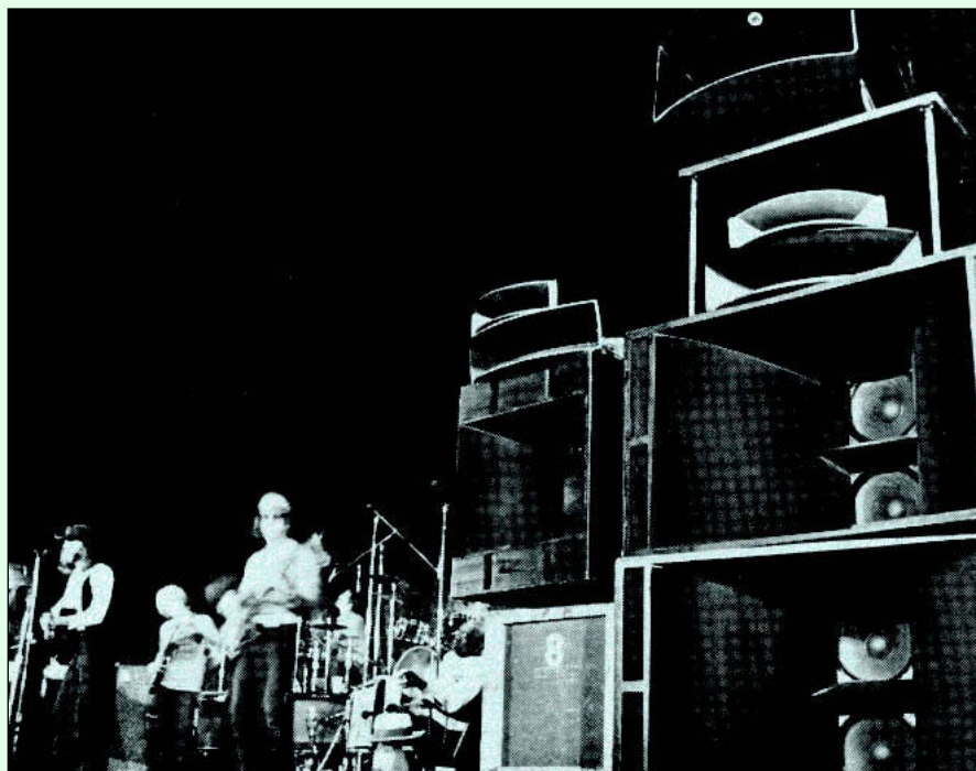
Fig. 7. Typical early-1970s horn-loaded system using ported LF horns, 90° radial horns with large-format drivers, and 90° radial horns with small-format drivers for augmenting the upper frequencies. A narrow coverage horn with a large format driver is used for long-throw coverage. (Photo, JBL)
