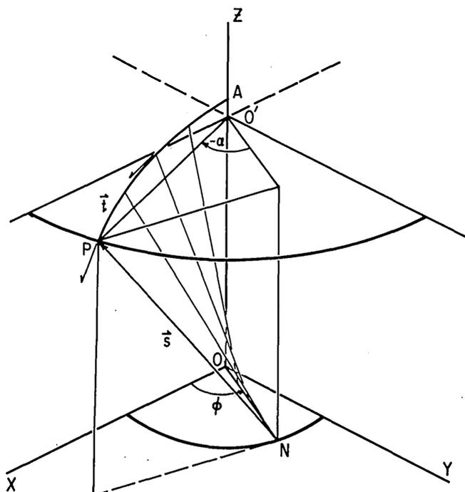
Fig. 8. A fan of skew lines, each having the same length from the elliptical arc  $PA$  to the line segment  $NO$ . Each skew line is the rectilinear generator for one of the members of the family of hyperboloids in the oblate spheroidal coordinate system. The vector  $t$  is the tangent vector to the elliptical arc, and  $s$  is the skew-line vector.
