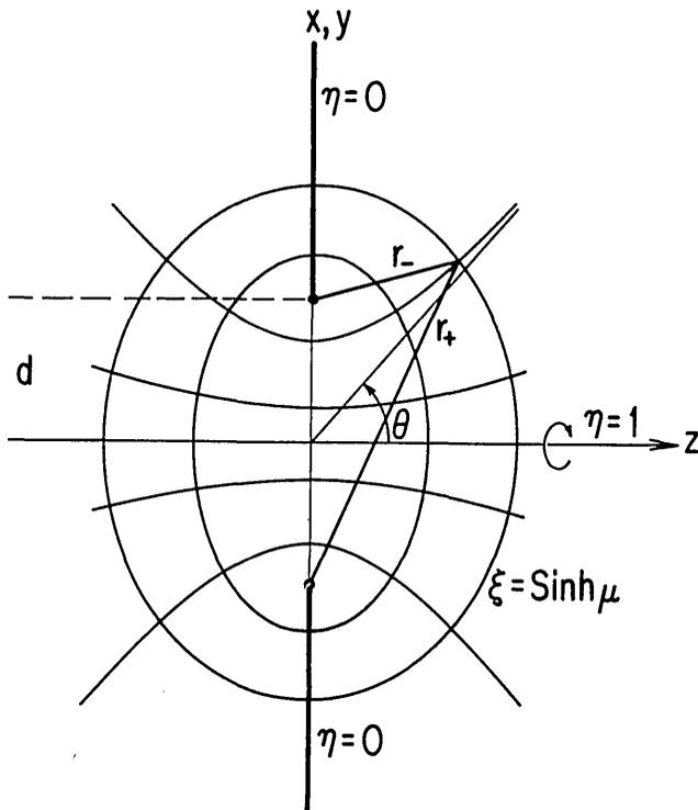
Fig. 1. Oblate spheroidal coordinate system.
