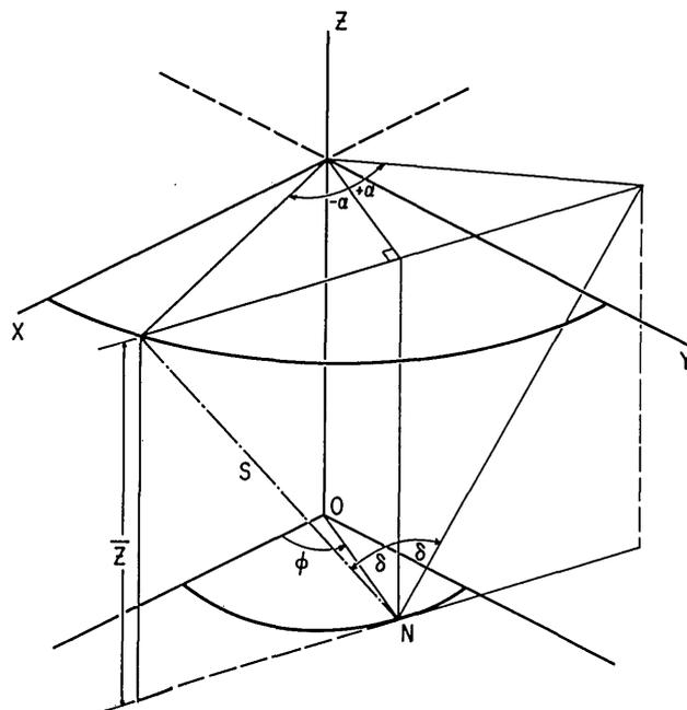
Fig. 6. The two possible twist orientations for the skew line  $S$ : a counterclockwise twist for  $+\alpha$  and a clockwise twist for  $-\alpha$ .
