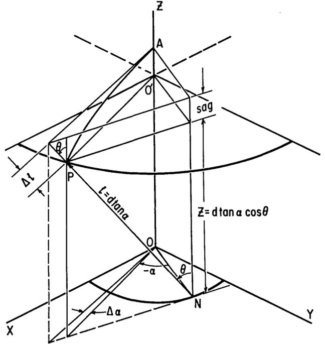
Fig. 9. The differential change in twist angle,  $\Delta \alpha$ , corresponds to the sag of the elliptical arc,  $PA$ , as measured along the skew line. This distance is given by  $d\xi/\eta - d\xi$ .
