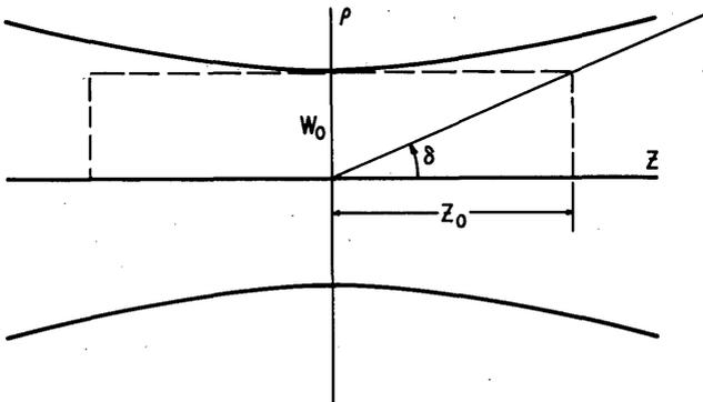
Fig. 3. Cross section of the hyperboloid generated by the rotation of a skew line about the z axis.
