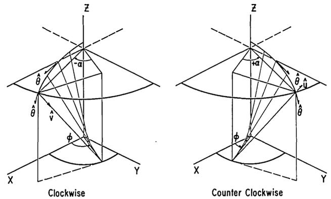
Fig. 10. Skew-line fans for a clockwise twist ( $-\alpha$ ) and a counterclockwise twist ( $+\alpha$ ), for discrete skew lines. The skew lines are denoted as the vectors  $\hat{v}$  and  $\hat{u}$ , and  $\hat{\theta}$  is the tangential vector to the elliptical arc. The figures are mirror images of each other.
