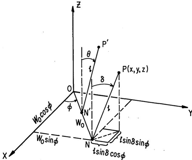
Fig. 2. Orientation of a skew line with respect to the z axis. The skew line,  $l$ , is shown for two possible deviation angles,  $\delta$  and  $\theta$ .
