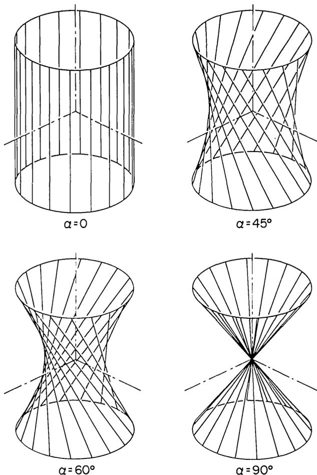
Fig. 5. Different ruled surfaces generated by varying amounts of twist of the rectilinear generator (skew line). For zero twist, the straight line produces a right circular cylinder. As  $\alpha$  increases, the figure becomes a hyperboloid of one sheet of increasing divergence until, in the limit of  $\alpha = 90^\circ$ , it is a right circular cone.
