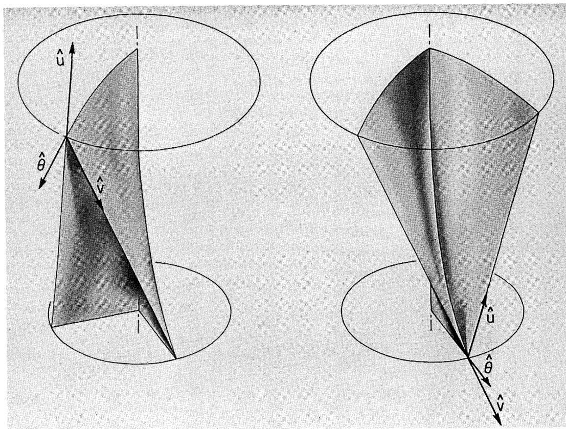
Fig. 12. Unit base vectors  $\hat{u}$ ,  $\hat{v}$ , and  $\hat{\theta}$  for a nonorthogonal coordinate system. The two conoids join in an elliptical arc in the left-hand drawing. Their junction in the plane of the waist is shown in the right-hand drawing.
