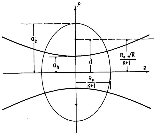
Fig. 7. Cross section of one confocal oblate ellipse and hyperbola. Their common foci are spaced at  $2d$ ;  $K$  is the conic constant of the ellipse, and  $R_e$  is the radius of the vertex curvature of the ellipse along the semiminor axis.
