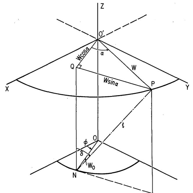
Fig. 4. Skew line projected onto a plane perpendicular to the  $z$  axis and a distance  $NQ$  from the plane of the waist.
