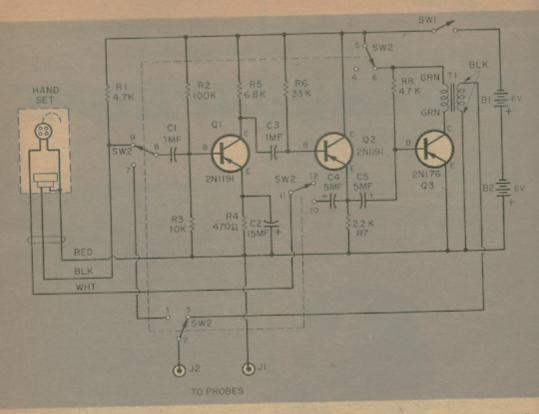
Transistor amplifier is heart of Terraquaphone, Talk-Receive switch (SW2) is shown in Talk (depressed) position. In Receive position, power transistor Q3 is switched out and current drain is only 10 ma.
