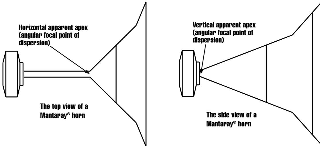
The planar sections do not provide quite as good a driver-loading characteristic as the EV's radial sections, but they are adequate for an 800 Hz crossover frequency, and provide superior vertical control with a more symmetrical mouth size.
