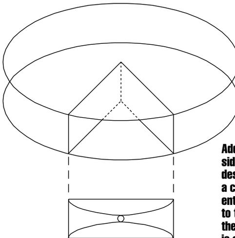
**Add straight sidewalls at the desired angle and a circular throat entrance to mate to the driver and the radial horn is complete**
