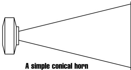
Variations using rectangular cross-sections and flat planar walls provided directional control at the expense of some wave-front distortion. Some of these variations no longer follow the strict definition of a conical horn since the expansion rate of the horn area is no longer a conical expression mathematically. The weakness of conical horns lies in their acoustical loading characteristics for the transducer, which is insufficient at the low-frequency end of its desired frequency range.
