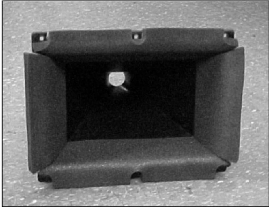
The mathematics that describes this design are not within the scope of this paper. However, as a point of information, the formula describing the cross-sectional area expansion rate of the throat section is in the form of a quadratic equation, hence the name Quadratic Throat. Its formula is as follows:
