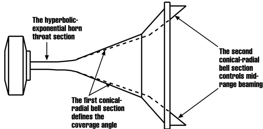
Having constant beamwidth in both the vertical and horizontal directions, and an unprecedentedly high directivity index, or Q-factor, these horns became the model for virtually all new horn designs for the next decade. Additionally, the horn loaded the driver well and as a result, sounded very good.
