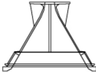
**An AutoCAD drawing of the 60-degree by 40-degree Quadratic-Throat Waveguide®**
