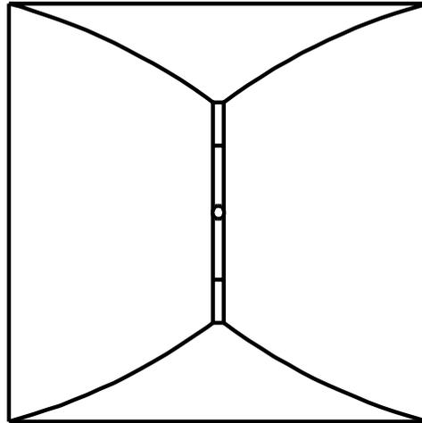
Since the design still incorporates the diffraction slot, and still has the differing apparent apices, the design still suffers from the same astigmatism as the Mantaray® horn.
