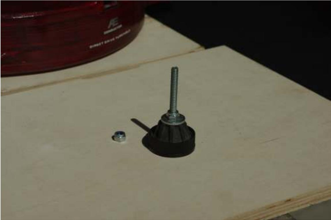
Photo of an adjustable mounting foot
