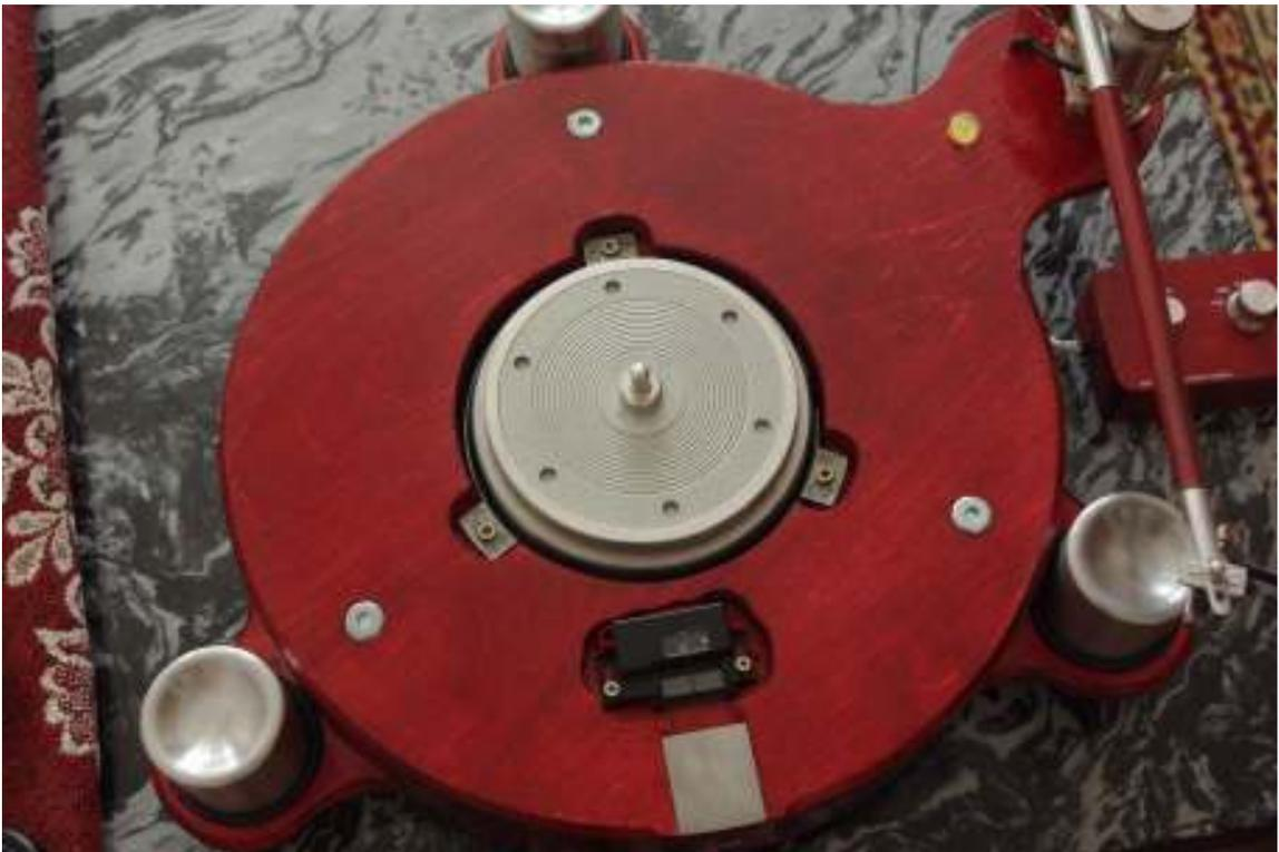
Top view of turntable with arm installed and leveling (bubble) indicator
