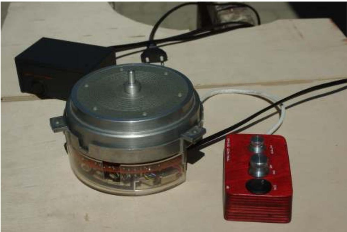
The Dual 701 motor assembly. Control circuitry is contained in the base of the motor.
