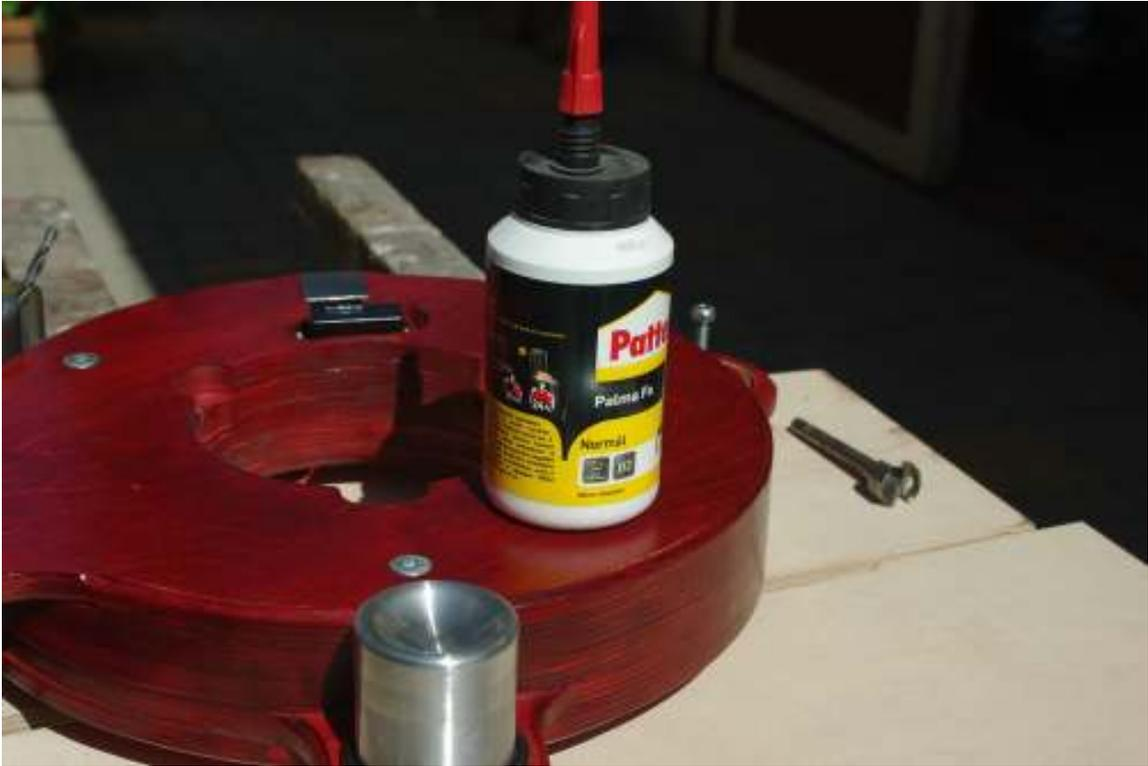
Adhesive used to hold the finished laminations together after being sanded. Staining was actually accomplished after this step.
