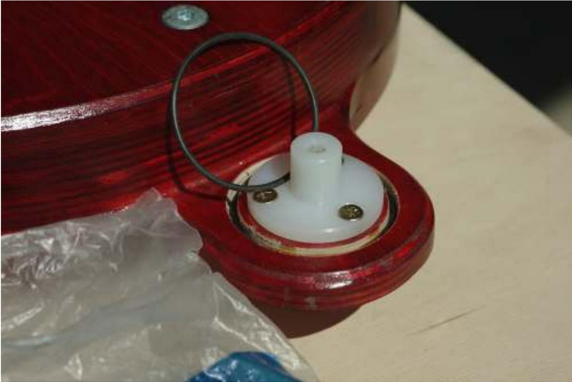
“O” ring before being placed in the slot
