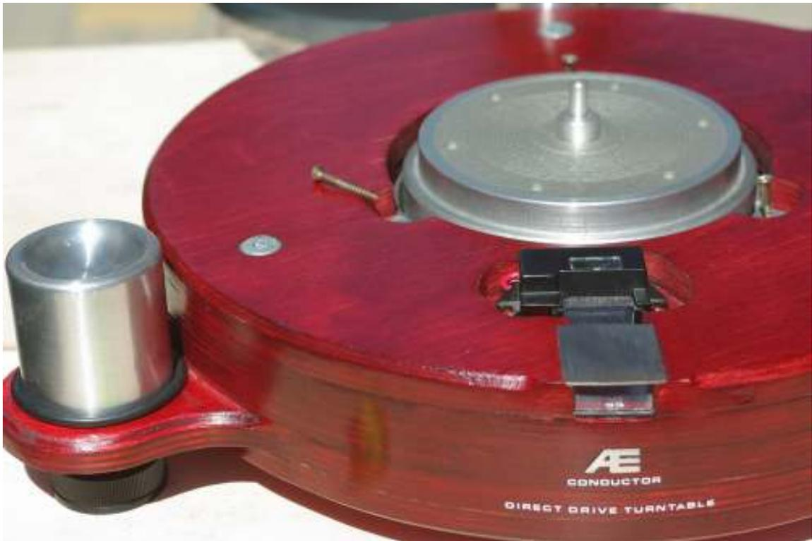
Detail for the speed/strobe indicator placement.
