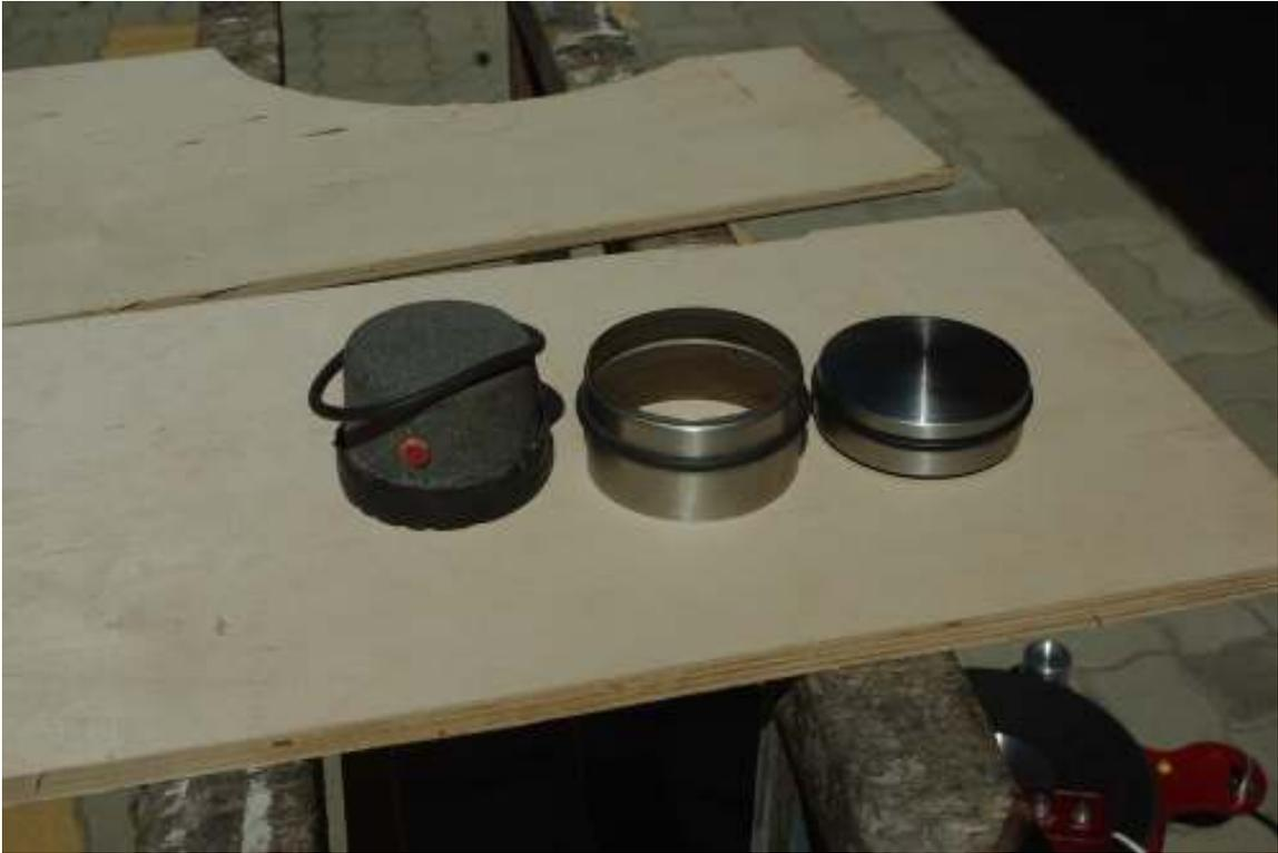
The door stop disassembled
