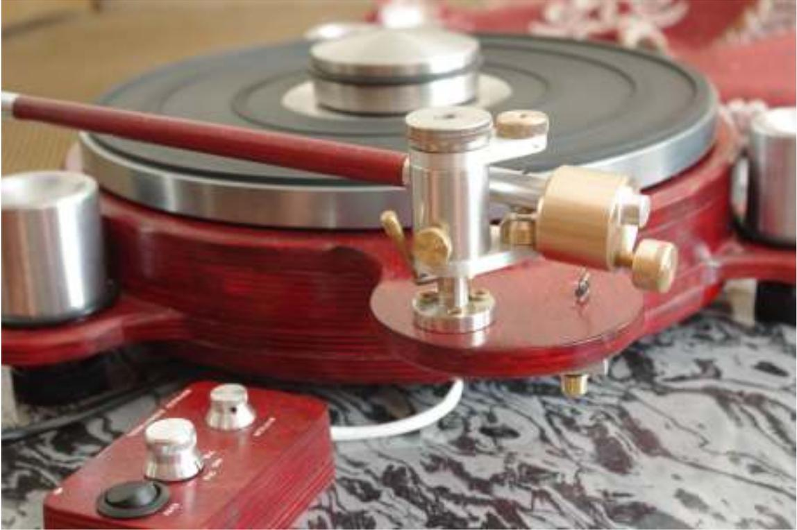
Side view of the tone arm and mount detail. Note the air gap between the arm and base
