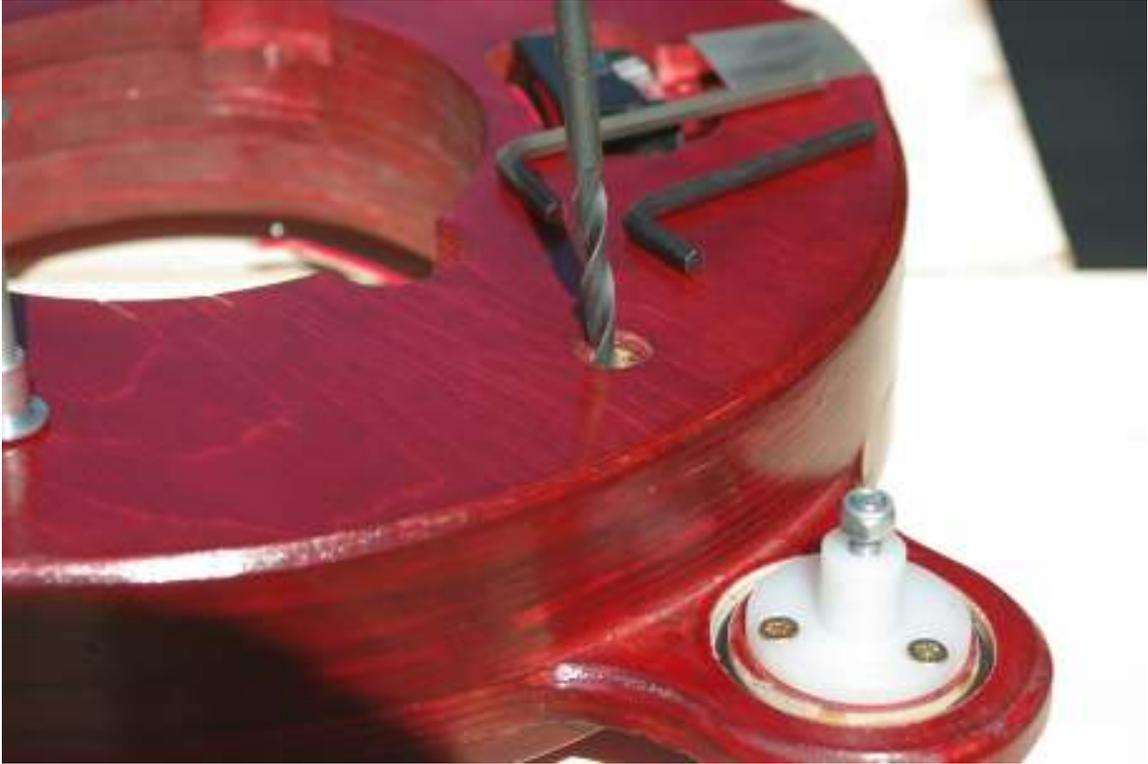
Drilling holes to secure the laminations together
