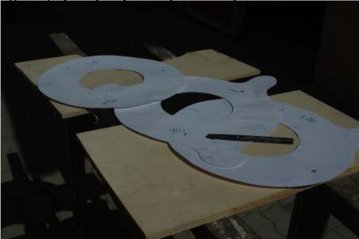
The first photo shows the templates used to cut the plywood sections for the finished base.
