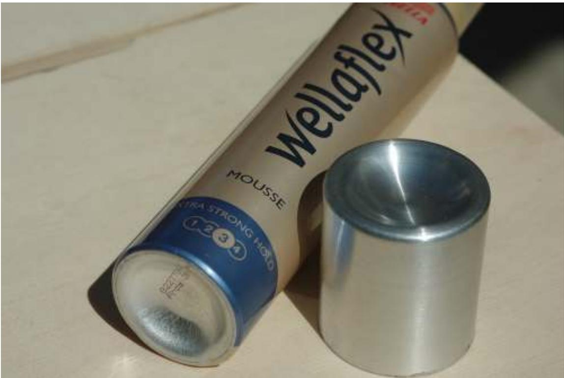
Source of the mounting feet supports – a cosmetic tube cut to size
