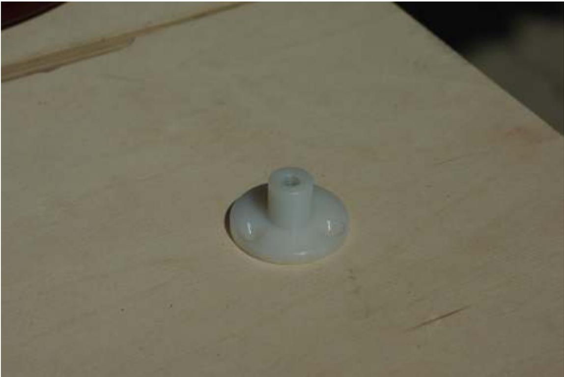
Photo of the sleeve for a mounting foot
