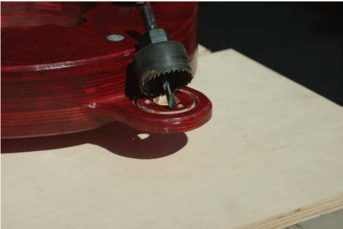
Method for making the circular slot for the mounting feet
