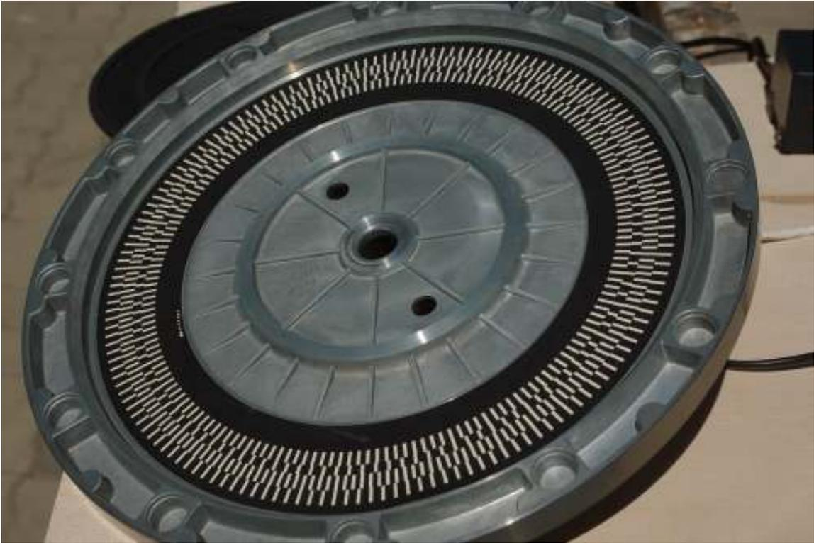
Bottom view of the Dual 701 platter. Note the strobe marks that are used with the speed/strobe assembly to indicate and verify the speed.
