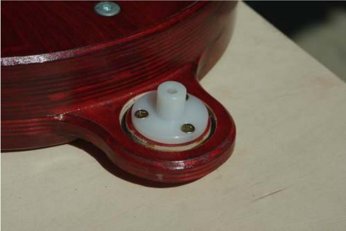
Mounting foot sleeve shown attached to the top surface of the support
