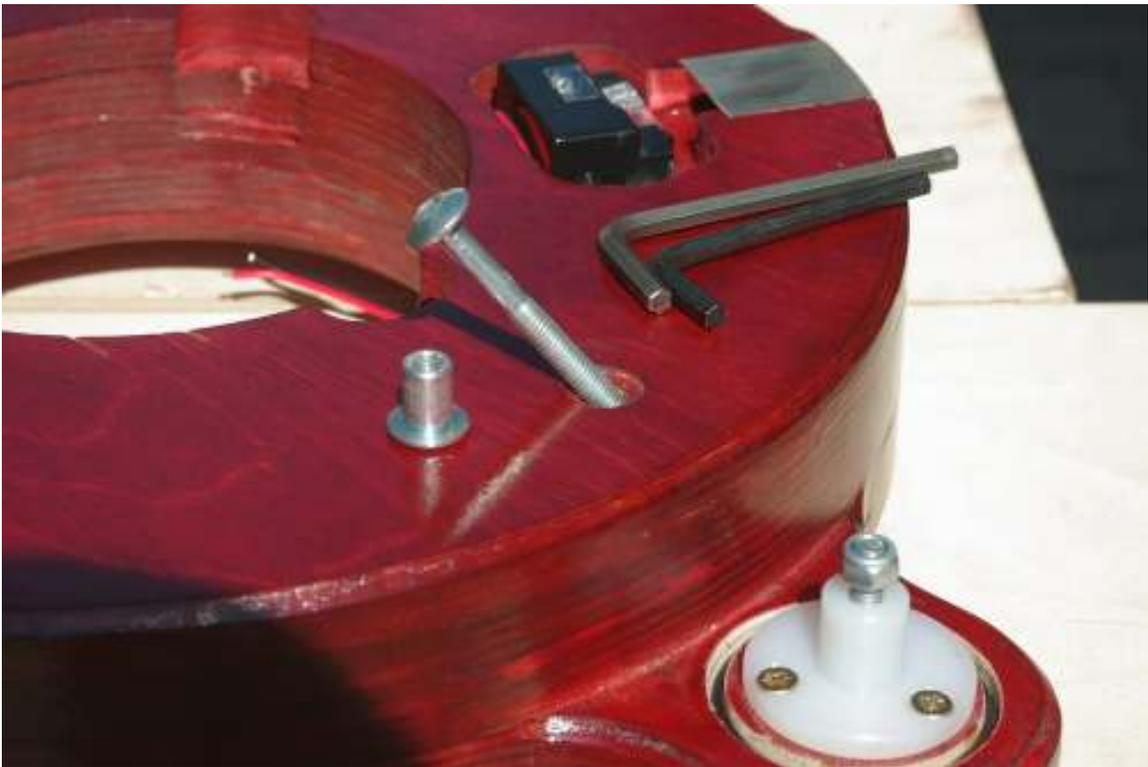
One of three bolts that secure the laminations
