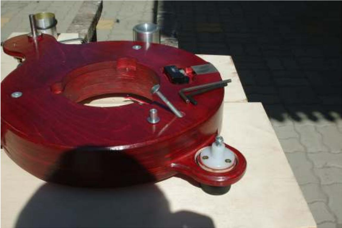
Another view of the bolts – three at approximately equal spacing. These bolts were used to hold the laminations together for sanding. The photo is after the sanding was done and laminations were stained.
