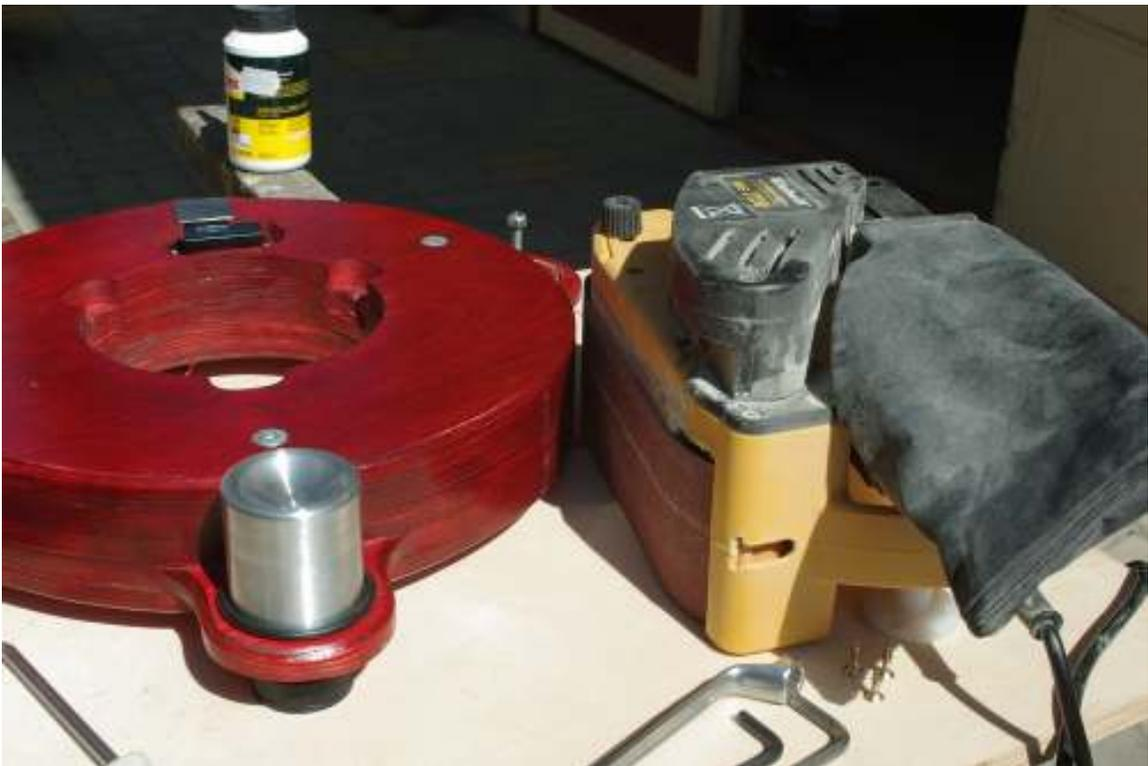
The type of sander used to smooth the cut out laminations
