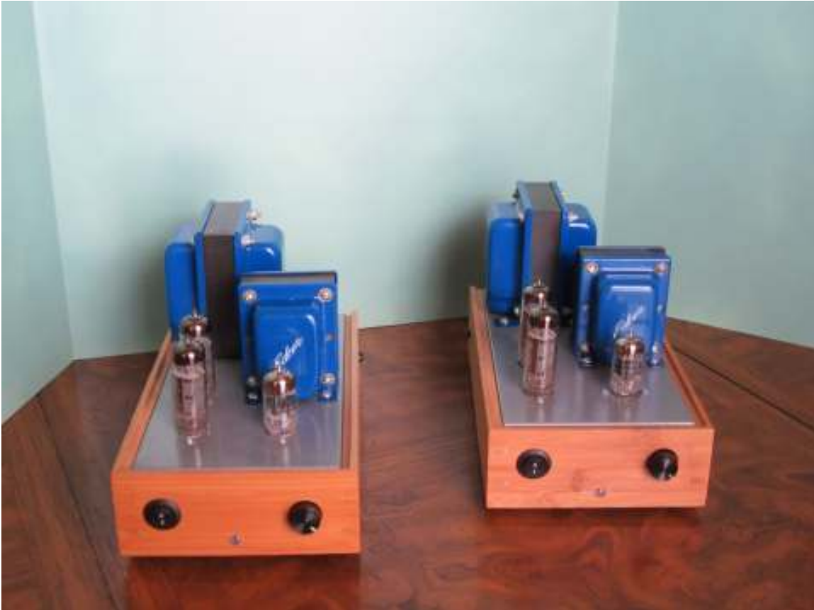
A Pair of Mini Blocks (the bigger transformer is the power one)
